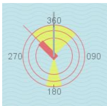
Bearing to mark: 360° Wind direction: 360° Compass-Course: 315°
