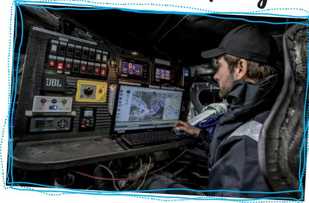
This is Boris in his small "office". Here he can make calls using a **satellite telephone**, send emails, receive weather data and navigate.
